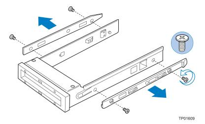
Figure 24. Removing the Rails from the Floppy Drive Conversion Kit Carrier
